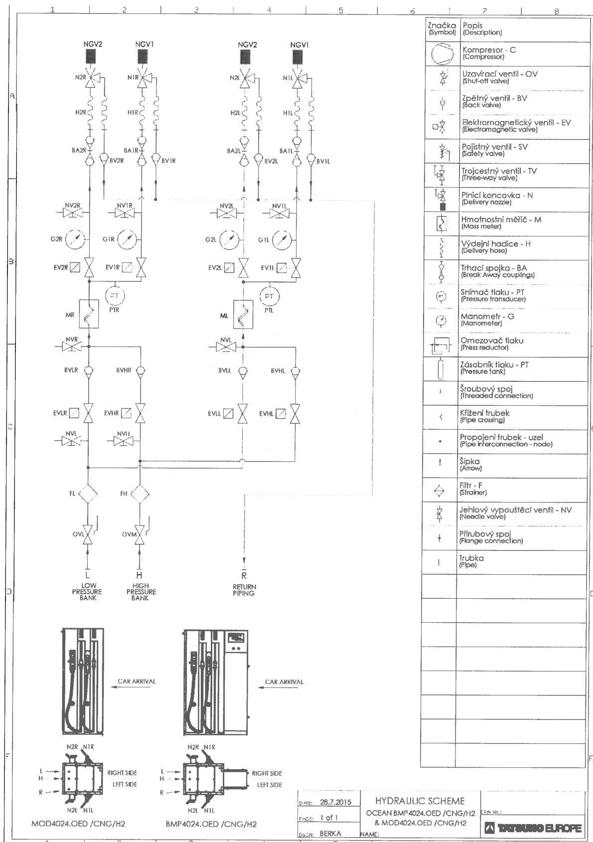
Figure 3: Hydraulic scheme for CNG dispenser with 3 banks:
