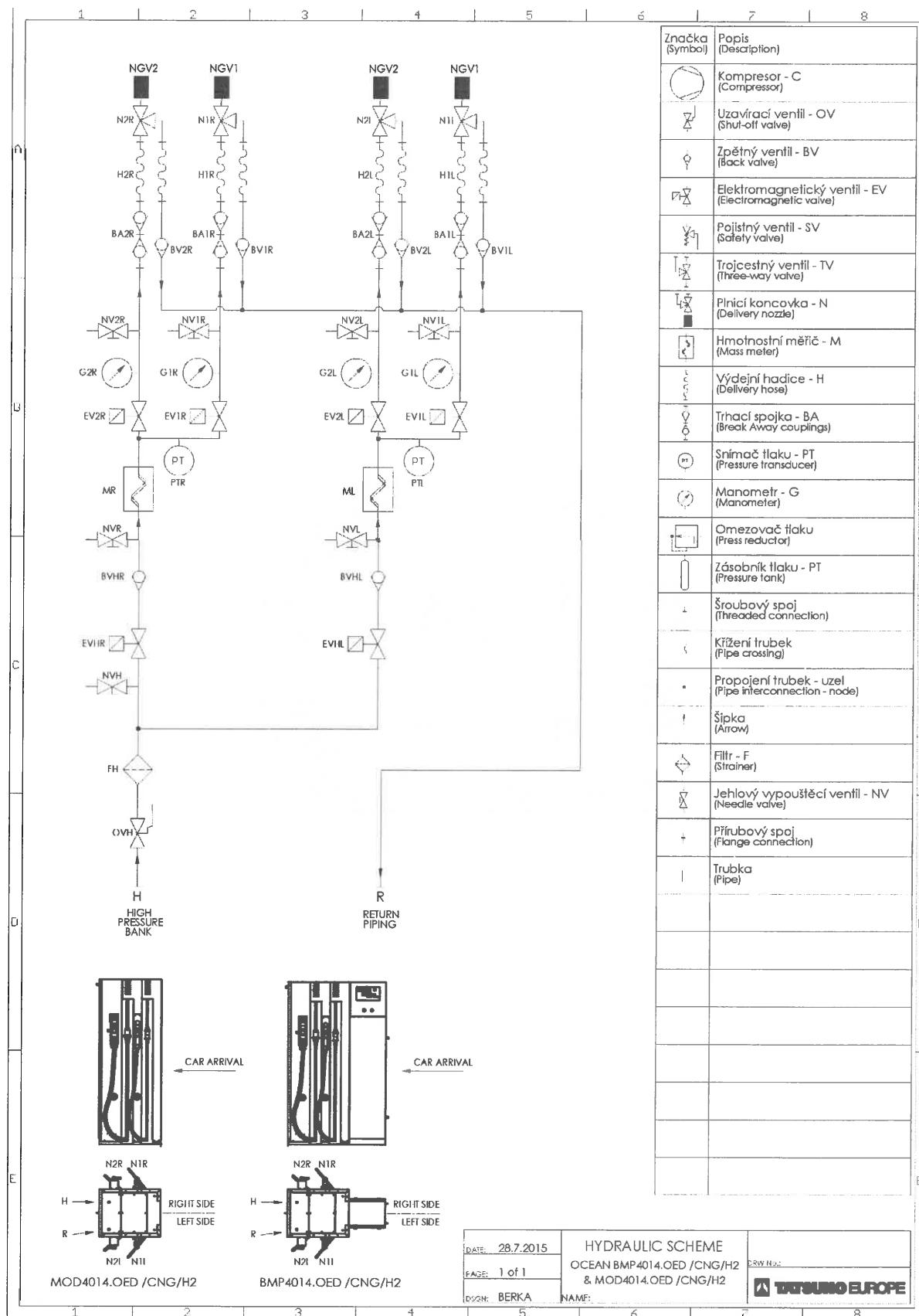
Figure 2: Hydraulic scheme for CNG dispenser with 2 banks:
