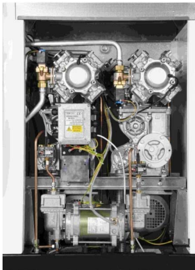
Fig. 28 – Dispenser without cover, side B
