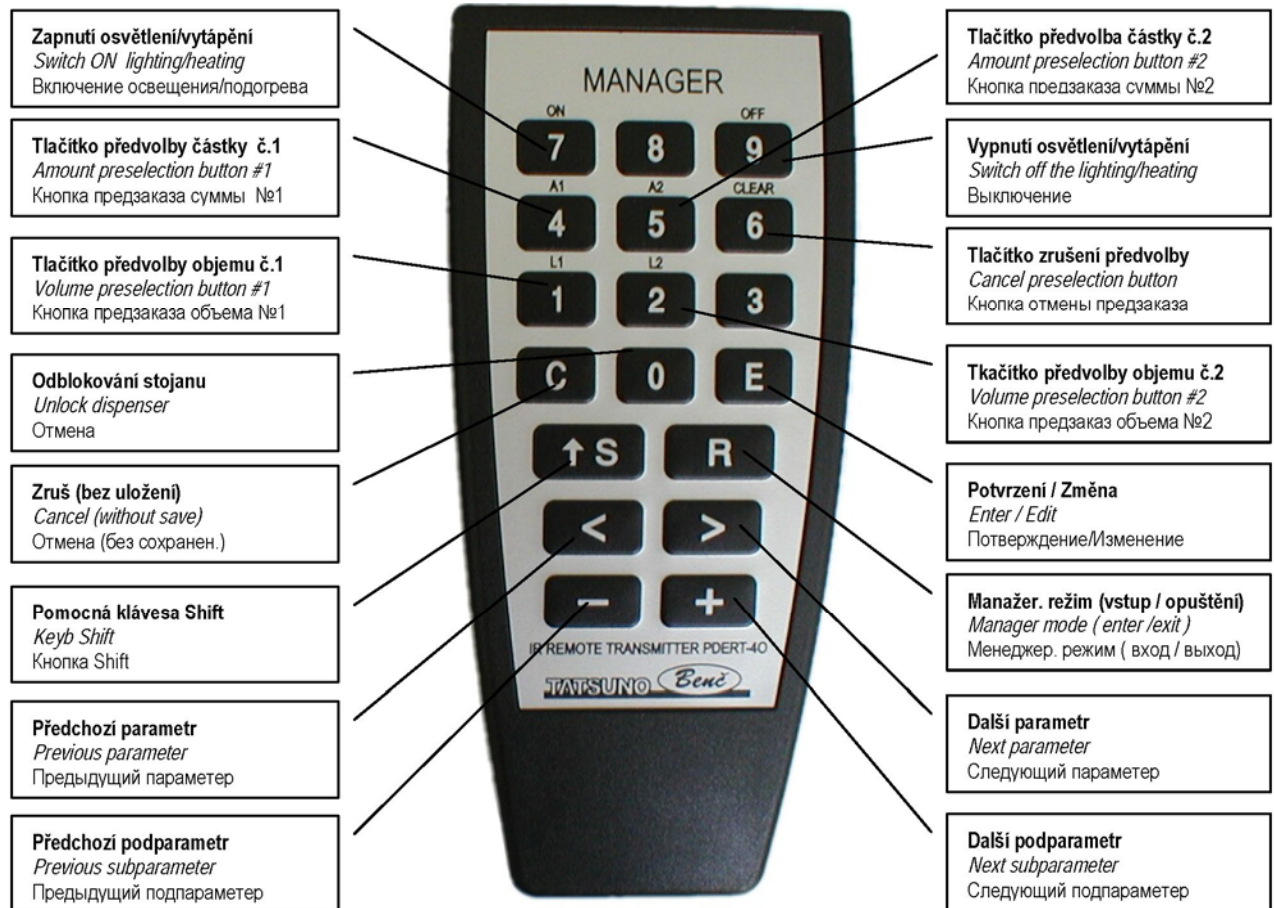
Fig. 20 – Description of keys on the remote controller PDERT-50
