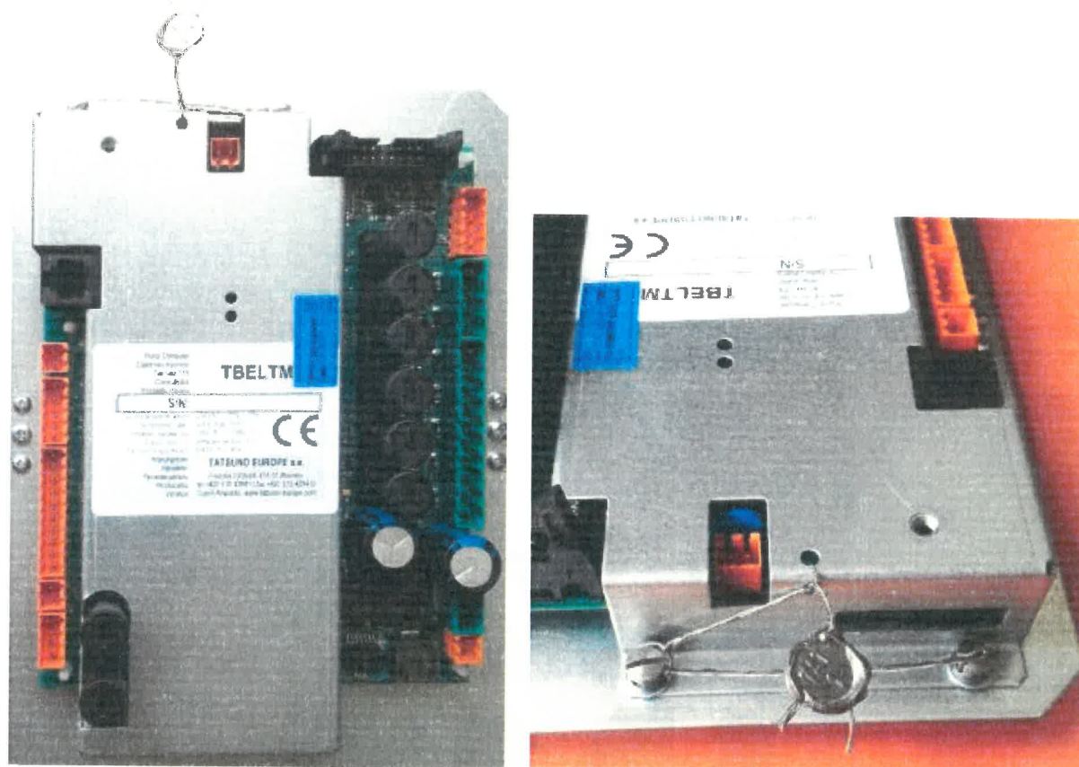
Picture No. 11: Sealing of the TBELTM calculator
