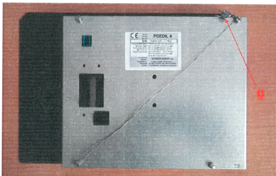
Picture No. 4b : Sealing of the totalizing indicating device with display PDEDIL V6
