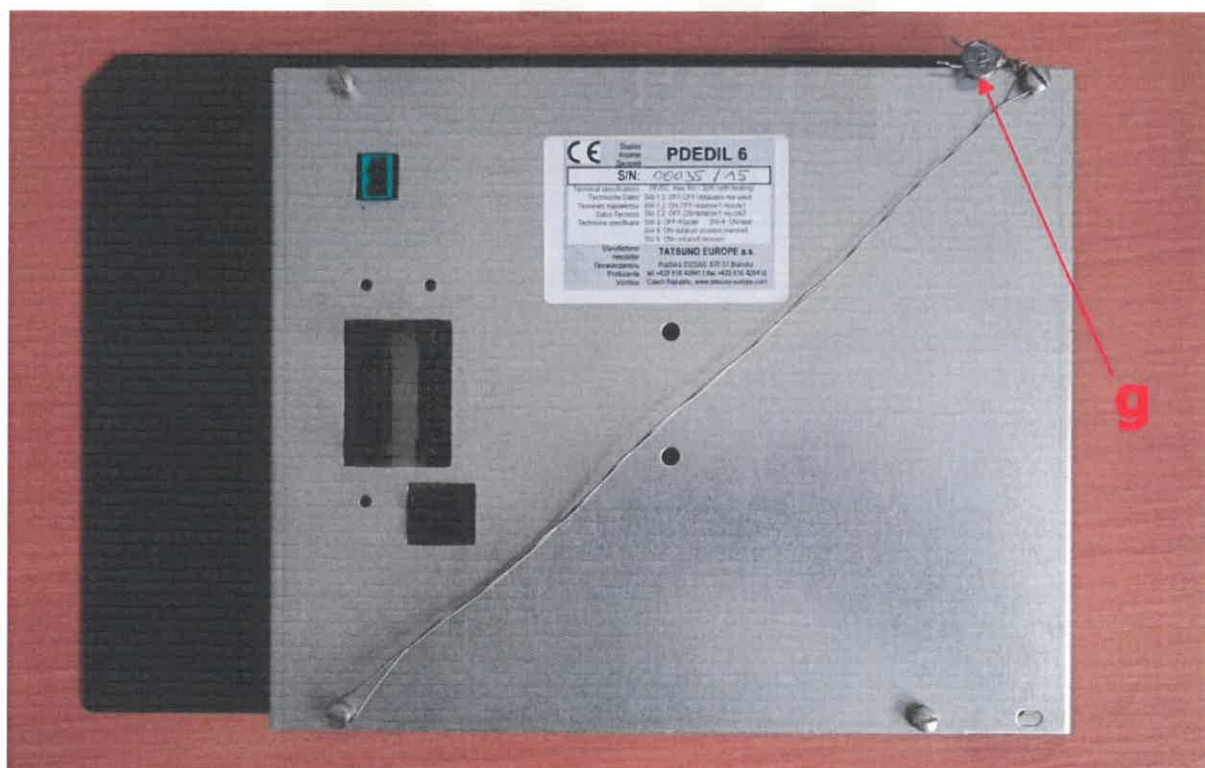
Picture No. 3b: Sealing of the totalizing indicating device with display PDEDIL V6
