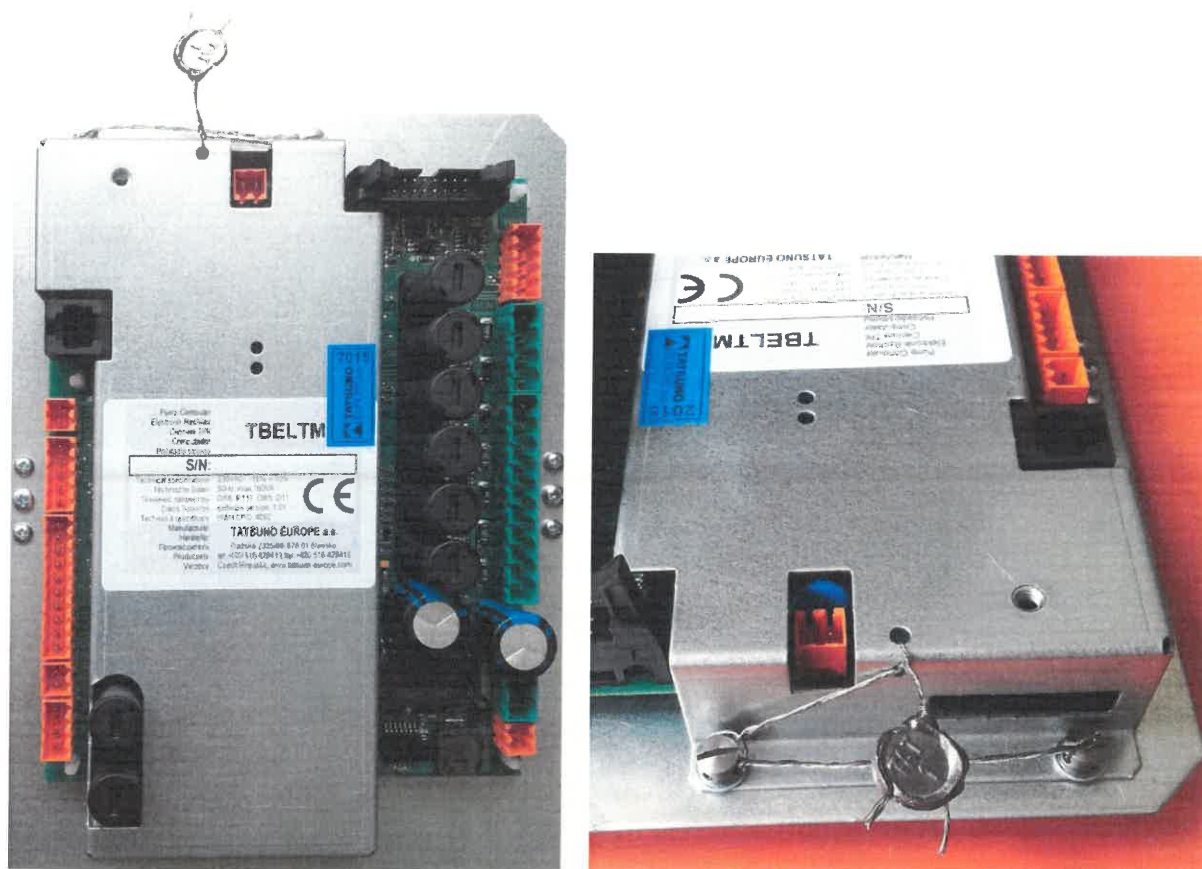
Picture No. 11: Sealing of the TBELTM calculator
