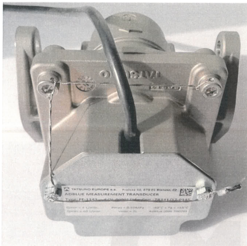
Picture No. 2c: The sealing of FF-1141 measuring transducer
